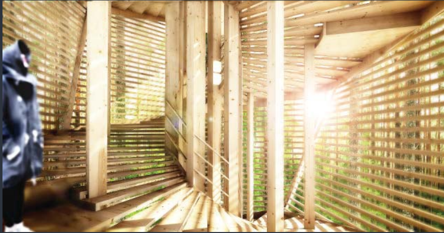
Figure 2.25 - The perspective shows how the it would feel to climb the stairs to the peak surrounded by the wooden slats. The slats allow light into the space to allow people to see without the need for artificial lighting which creates a more natural feel and blends into the surroundings better.
