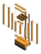
Construct wall system using studs on a flat horizontal surface allowing for a 2'-0" by 2'-0" opening for the window.
