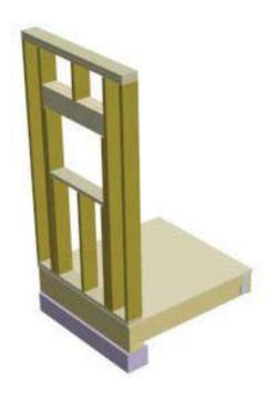
3k) Take wall assembly, place on top of subfloor and nail to plywood. Fashion temporary racing to hold the wall up for assembly of roof and finishes.
