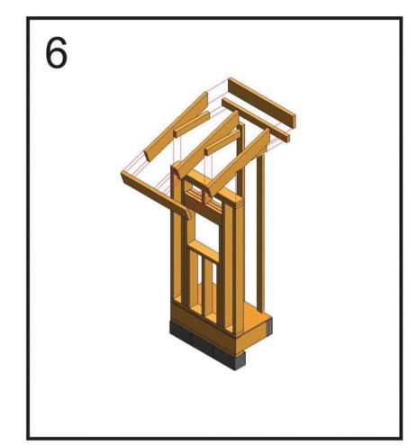
Create a birdmouth notch on the underside of each roof rafter to allow the top plate of the wall to join with the rafters creating a 4"/12" drop in the roof. (3" notch up to a 6" notch deep)
