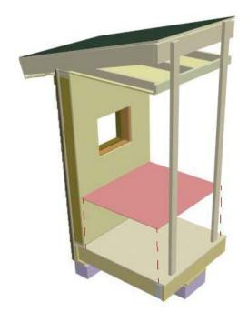
6b) Adhere nailing strips to subfloor, place carpet pad, then carpeting on top of that.
