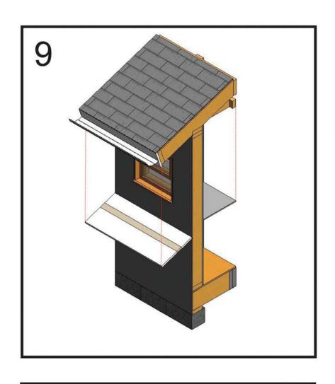
Position and fasten soffit and vent onto the underside of the roof overhang.
