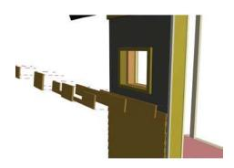
7c) Place and nail in freeze board between the top clapboard and the soffit board.
