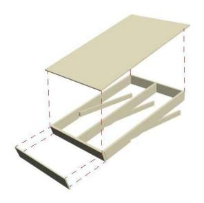
4e) Place and nail 4' long 1x10 fascia board to exterior face of roof joist.
