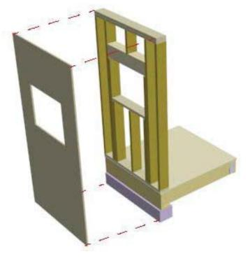
3l) Place  $\frac{3}{4}$ " plywood sheathing on exterior face of wall and nail to studs.
