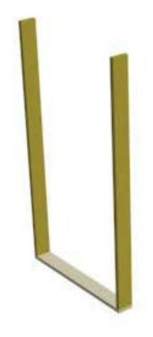
3b) Place and nail in (2) common studs on the outside edges of sole plate. Use 3" framing nails.
