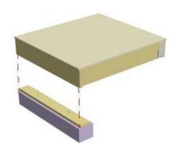
2e) Place floor system and nail to rim joists, then place ¾" plywood sheathing on top of floor and nail down. Use 2" framing nails.
