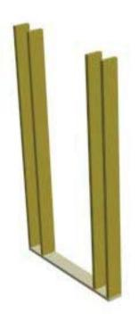
3c) Place and nail in (2) king studs 7  $\frac{1}{2}$ " inside of the common studs.
