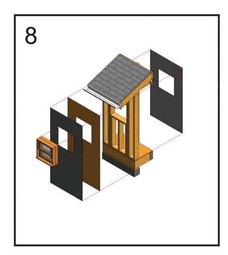
Position and fasten gypsum wall board to inside of wall leaving a 2'-0" by 2'-0" opening for window.
