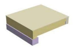
2f) Place floor on top of sill plate aligning the outside edge of rim joist with the exterior edge of the sill plate. Place CMU block with 2x member under the back rim joist for support.
