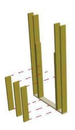
3e) place and nail (2) 3'3  $\frac{1}{2}$ " cripple studs directly to the inside edge of the jack studs then place and nail another directly centered between the 2 others.
