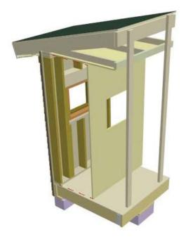
6b) Place and screw GWB to interior face of wall.
