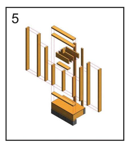
Construct wall system using studs on a flat horizontal surface allowing for a 2'-0" by 2'-0" opening for the window.
