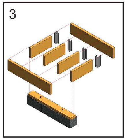
Position and fasten floor joists to rim joists using joist hangars.
