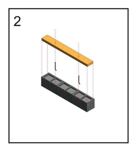
Set anchor bolts into still wet concrete approx. 12" from each end of wall.
