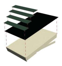
4f) On top of roof felt nail down asphalt shingles starting from the bottom and working up, making sure to overlap the shingles.
