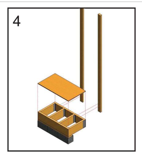
Position and set subfloor sheathing to floor joist platform.
