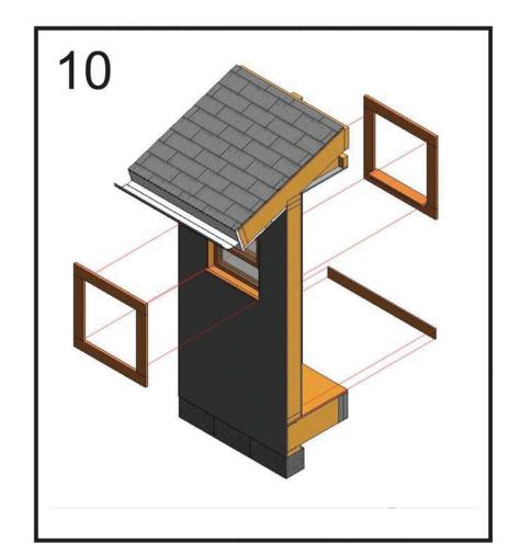
Position and fasten window trim and sill to the perimeter of the window opening both on the exterior and interior.
