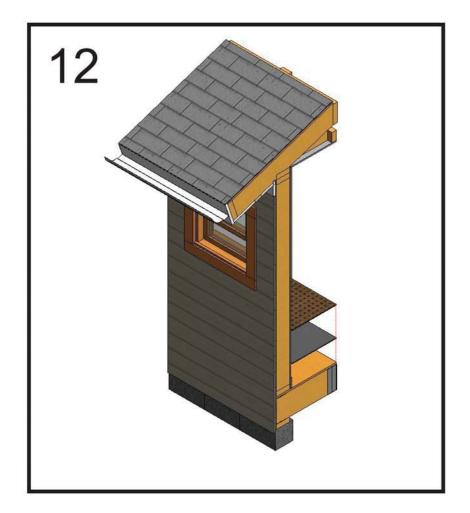
Position and fasten carpet pad to floor sheathing using construction grade staples.
