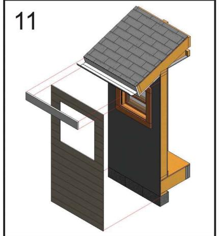
Position and fasten each length of clap board starting at the bottom with a starter strip and working up to the roof.
