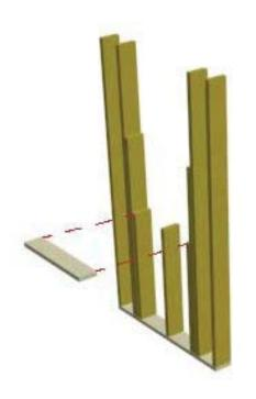
3f) Lay 2' 2x6 sill plate for window along the top of the cripple studs and nail in place (3" framing nails)
