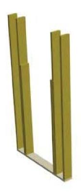
3d) Place and nail (2) 5'5  $\frac{1}{2}$ " jack studs directly to the inside edge of king studs
