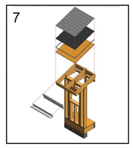
Place plywood roof sheathing onto roof rafter system.
